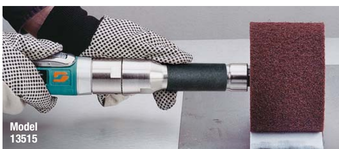
13515 Dynastraight® sets grain pattern in stainless steel.
