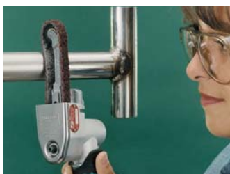
Clean and finish using non-woven nylon belts.
