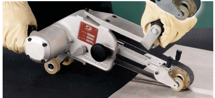
Place 11486 Dynabelter handle at 45° angle from belt housing to increase grinding pressure. Pull tool toward operator for faster material removal.
